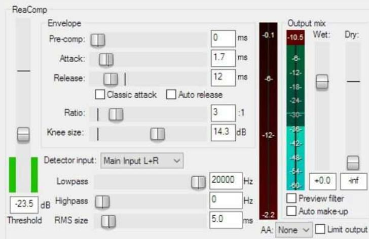
A compressor 'compresses' the loudest parts of your recording to make them more consistent with the rest of the recording. This in turn allows you to raise the overall volume of the recording without the loudest parts peaking.
